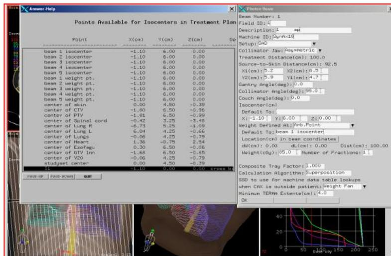
**Figure 4-** TPS preliminary data set to design and modeling the radiation beam of patient with XiO
