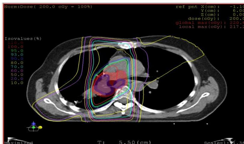
**Figure 2** – Three dimensional structures outlining external structures (surface of the patient), target volumes and risk organs taken from XiO
