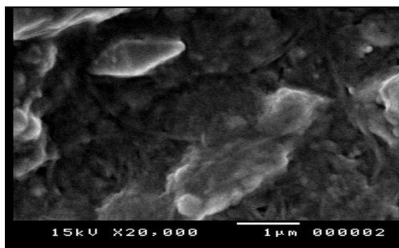
**Plate 2:** Scanning electron micrograph of crystal and spores of *thuringiensis* subsp. *Kurstaki* HD-1 (X20, 000)
