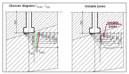
Fig. 6 and 7 Stresses diagrams (left) and instable zones (right).
