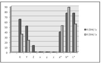
Chart 4. The experimental results of tri stimulus values, chromaticity coordinated and CIELAB coordinates for Kallmet red wine obtained according to CIE 1964 (x, y) color system (CIEXYZ) and CIELAB coordinates.
